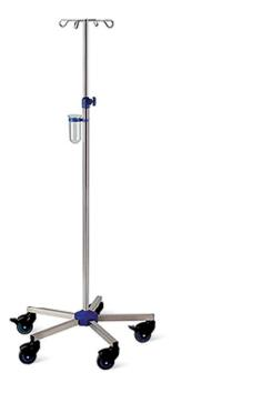
Structure made of telescopic AISI 304 stainless steel tube, diam. 25/18 mm, adjustable in height by screw from 1350 to 2150 mm.
